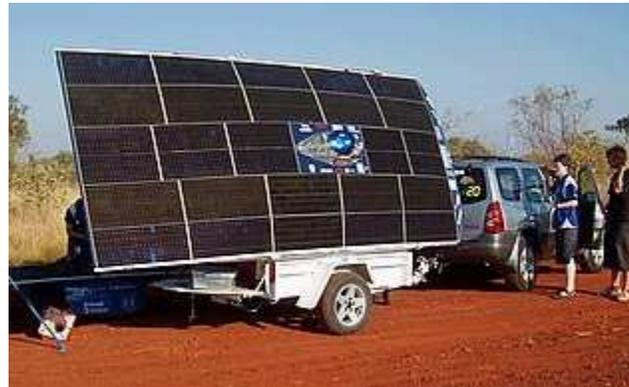
The most important job was to point the solar array of the car directly at the sun in order to put electrical charge into the batteries. The race rules do not allow any other method.
