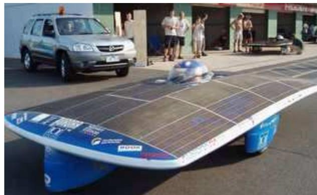
Anyway, we had our own stuff to do. Our new battery pack needed charging and installation for the first time. Jack had the task of setting suspension heights with the change in vehicle weight. The solar array needed a careful clean from the dirt it collected on the trip from Darwin. Finally we were able to get Andris out in the car for eight cautious but pretty smooth laps of the track.
