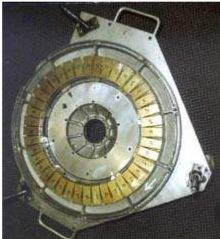
Wheel motor with surface mount magnets
