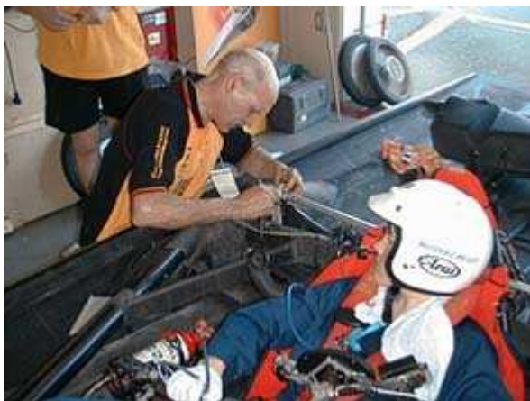
Fixing the broken panhard rod bracket
