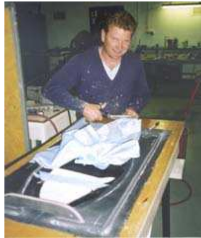
Darren Trafford building a new driver's entry hatch
