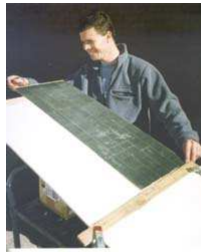
Matt O'Reilly checking a galium arsenide cell Gochermann solar panel
