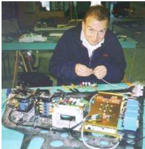
Brad Trewin building the main electrical tray
